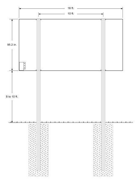
Once you have verified the positions of the posts and the size of the footings, you are ready to dig your holes, pour your concrete, and set your posts. There are several techniques for ensuring proper alignment of the posts. Typically installers will construct a temporary wooden support frame to hold each post in place while the concrete sets. Having plumb posts in the proper position is the key to a smooth mechanical installation.
